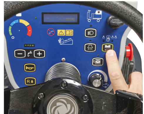
Brush deck/squeegee lowers automatically, minimising operator effort
